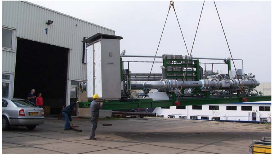
Metering skid being taken out of the assembly halls for packaging and subsequent delivery to customer
